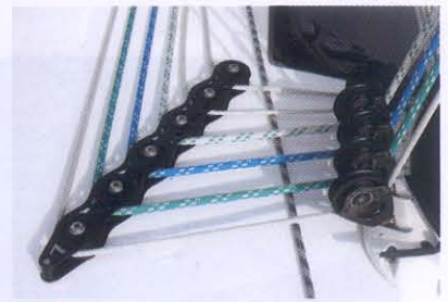
Above and below: keeping things tidy – lines led neatly aft from the mast base and a flush-mounted swim ladder that extends from the transom
