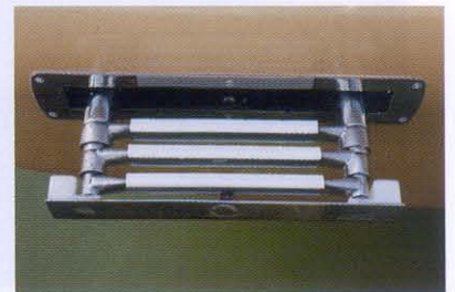
Above and below: keeping things tidy – lines led neatly aft from the mast base and a flush-mounted swim ladder that extends from the transom
