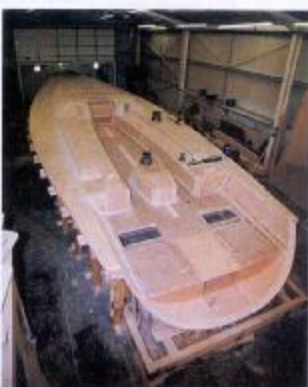
Above: hull and deck mould plugs near completion at Colvic
