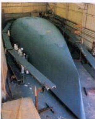
Above: hull and deck mould plugs near completion at Colvic
